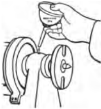
FIG. 76. — OILING SPINDLE OF A MACHINE.
